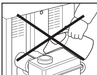
DO NOT FILL WITH FUEL OR LUBRICATION OILS WHILST ENGINE IS RUNNING
